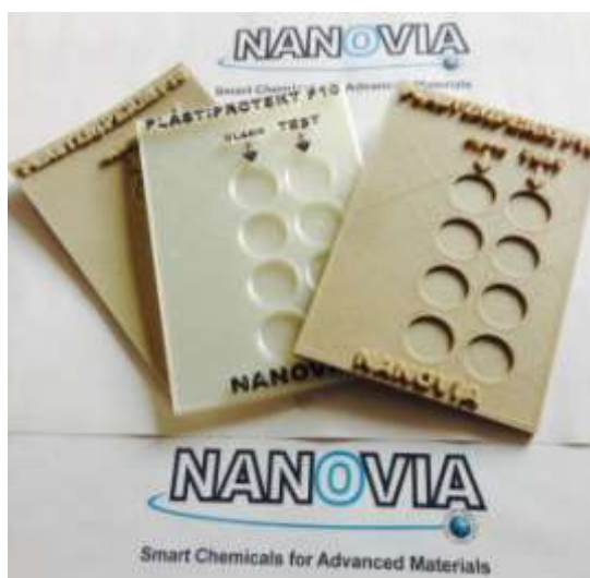
Right picture: Natural PLA blank vs treated with water and oil. (12 hours drying after solution mop application)
